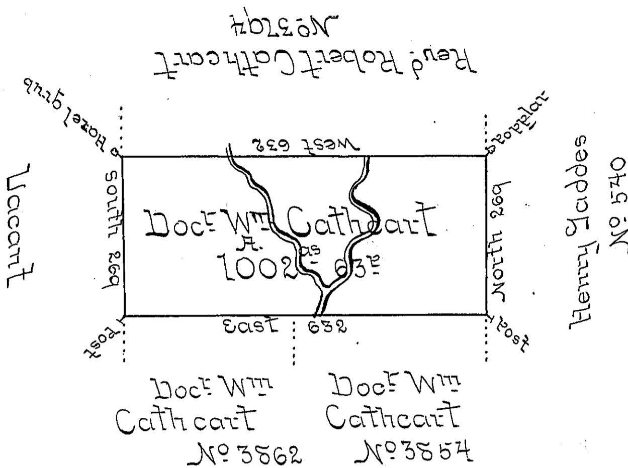
The Draught of Tract of Land ~~situate~~ situate on the waters of Stump Creek in the late Purchase in the County of Northumberland Containing One thousand Two Aces & Sixty three Perches with the usual allowance of Six P.C for roads Survey'd on the 19<sup>th</sup> Day of June 1793 in Pursuance of a Warrant No 3554 Granted to Doc<sup>t</sup> Wm Cathcart bearing Date at Philada May 6: 1793.
